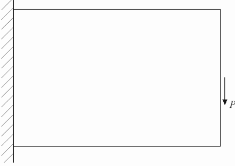
Fig. 1 Design domain and support conditions for example 1.
